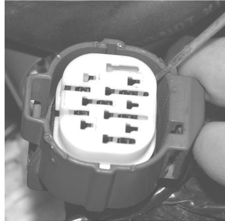
5. Remove the white pin protectors from BOTH plugs by using a screwdriver, as shown on the right. Note the orientation of the pin protectors.
