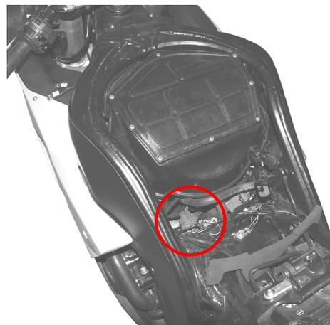
4. Depress the release tang (see at the left side of this picture) and disconnect the coupler. You may need a flat head screwdriver to get the coupler apart.
