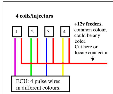
1. Locate +12v wire to ignition coil/s or fuel injectors (normally the same color for all coils/inj).
