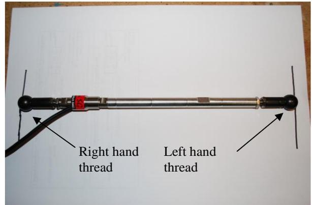
Cut and install sensor and confirm same length as the stock rod. SG sensor has Magic Threads, can take both left and right hand bolts in the same hole.
