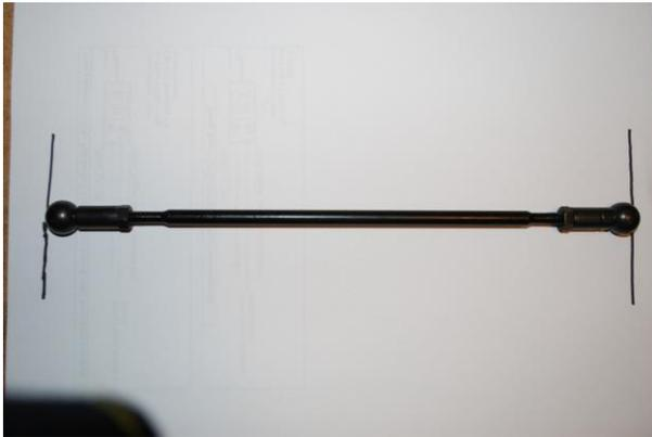
Remove stock shiftrod and measure.
