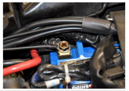
Use the supplied washer between the holder bracket and the mudguard.
